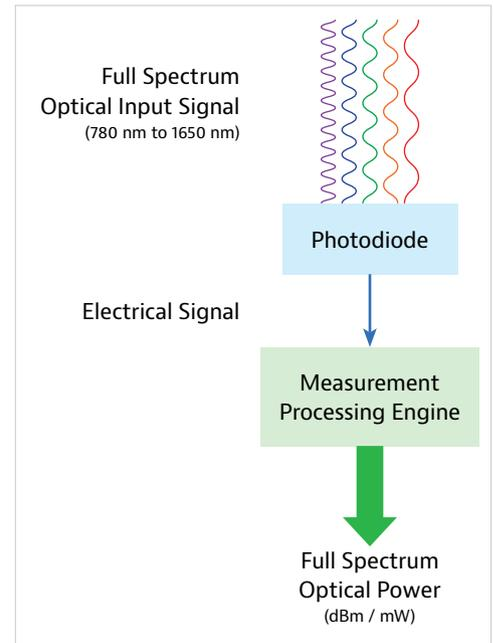
Figure 1: Broadband Optical Power Meter Schematic
