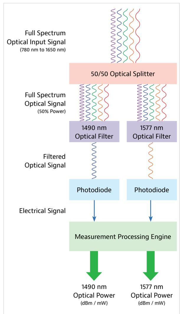
Figure 2: Selective Optical Power Meter Schematic
